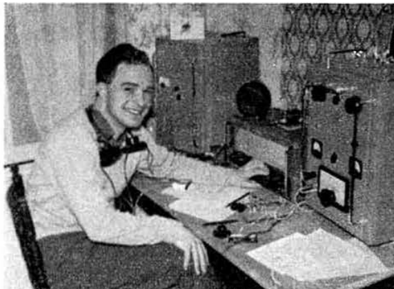
G3NHL operating GD6UW , the Cambridge University Wireless Society's DXpedition station in the Isle of Man, in April 1961. The transmitter was a Labgear LG300 and the receiver an Eddystone 888A.
